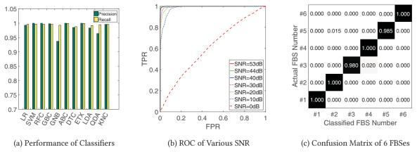
Figure 11: (a) describes the precision and recall of 11 common supervised learning algorithms; (b) describes the ROC curve of SVM classifier under different SNR conditions; (c) describes the confusion matrix of 6 FBSes.
