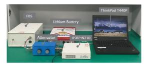
Figure 9: Lab Environment Experiment Setup.
