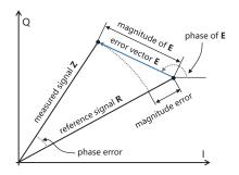
Figure 3: Definition of Modulation Errors.
