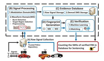
Figure 6: Working Flow of FBS1euth. The black arrow (left) indicates the procedure of processing raw FBS signals collected by the acquisition devices when FBS is committing the crime. The blue arrow (right) indicates the procedure of processing raw FBS signals collected by the police when FBS is caught.
