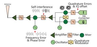
Figure 5: Structure of Superheterodyne Transmitter.
